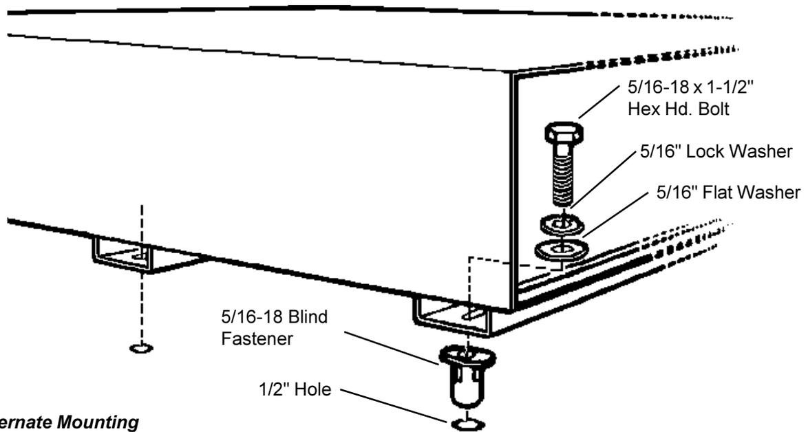
Figure 3. Alternate Mounting
